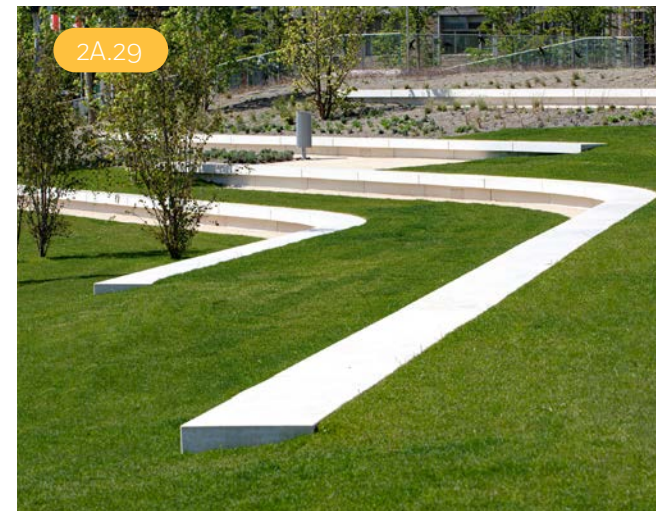
Concrete seat walls within the park landscape can be clever ways to provide park seating, but double as utility hook ups for vendors during events. Image credit Architonic.
