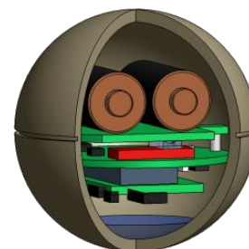
Aluminum core containing instrumentation and battery power.
