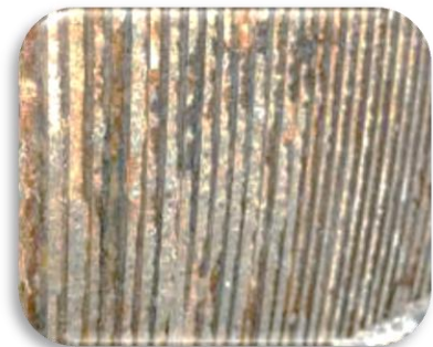
Heavily corroded and broken prestressing wire
