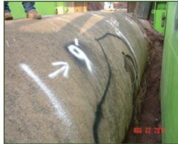
Damage concentrated in 9' section
