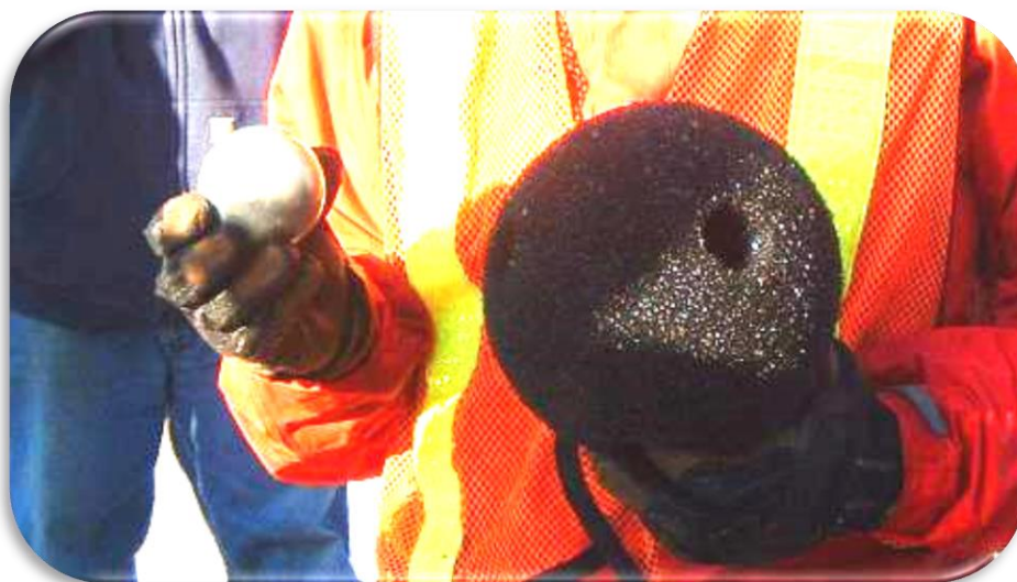
Aluminum core and outer foam protective ball.
