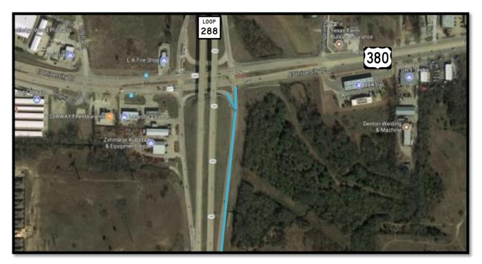
• ITS met with TxDOT Denton and TxDOT Dallas to begin process of adding turning improvements. TxDOT has included these improvements in the new maintenance contract. This exit ramp is included in the full depth concrete repair project scheduled to let on March 7, 2018. The work on widening/improving this ramp will likely begin in late April or early May.
