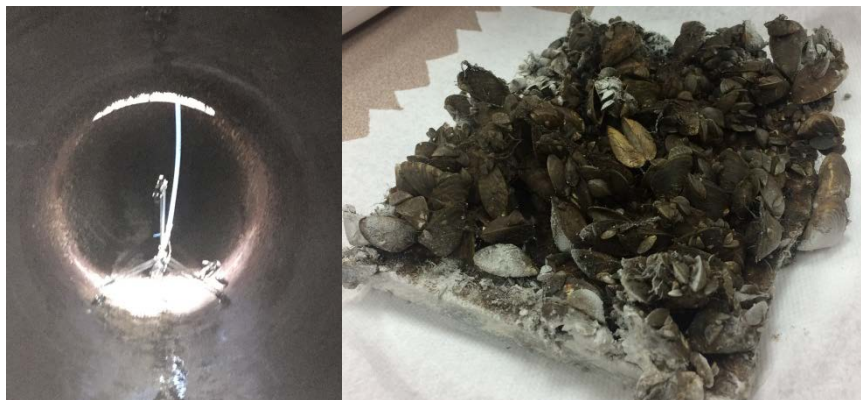
Figure 2-10: Hydroblasting the Raw Water Lines (Left) and a Fouled Pipeline Coupon (Right)
