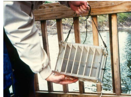
Figure 3-8: Example of a Substrate Sampler
