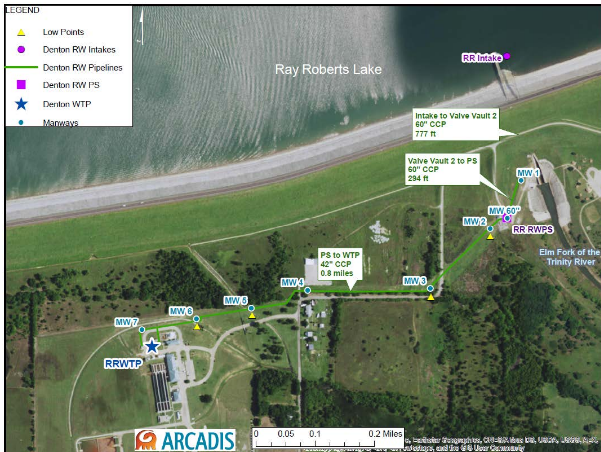
Figure 5-1: RRWTP Raw Water System
