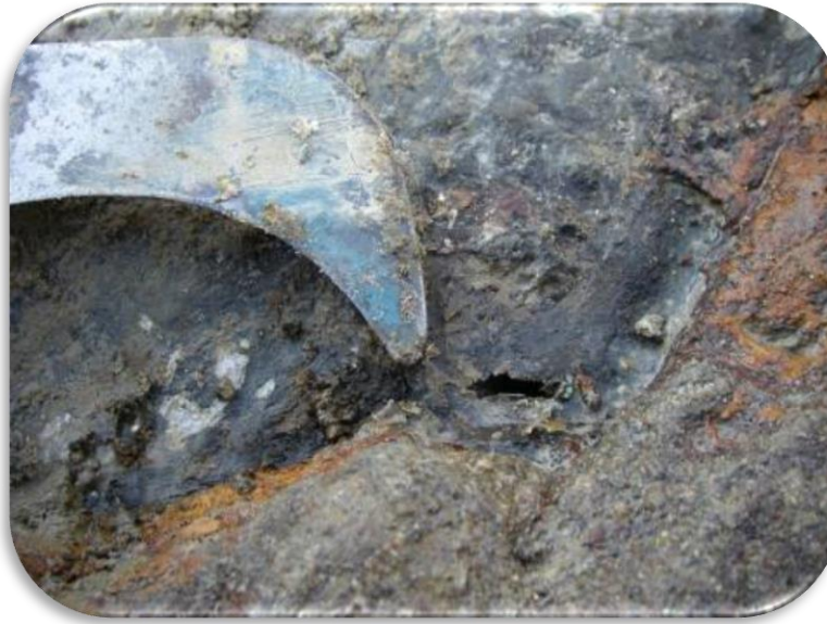
35 gpm leak at 1/4-inch slit in the steel bell joint of the PCCP
