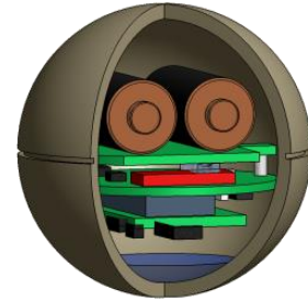
Aluminum core containing instrumentation and battery power.
