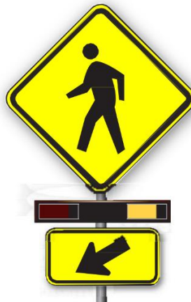
Figure 24 – Rectangular Rapid Flashing Beacon (RRFB) Source: TxDOT
