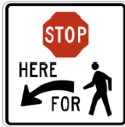
Figure 15 - Example of “STOP HERE FOR PEDESTRIANS” Sign
