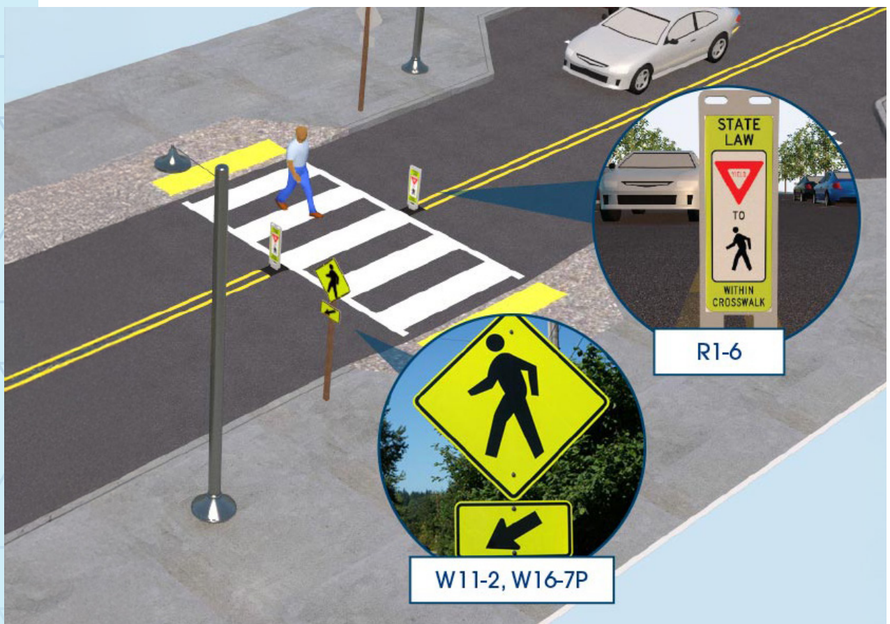
Figure 4.9. Improving Signing and Visibility at Signals Example
