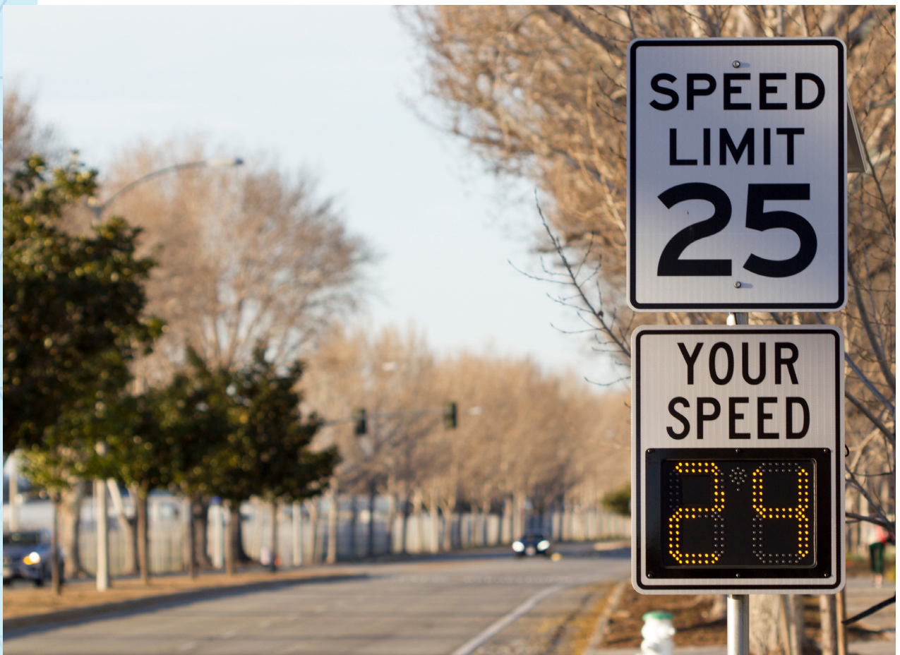
Figure 4.13. Dynamic Speed Feedback Sign Example
