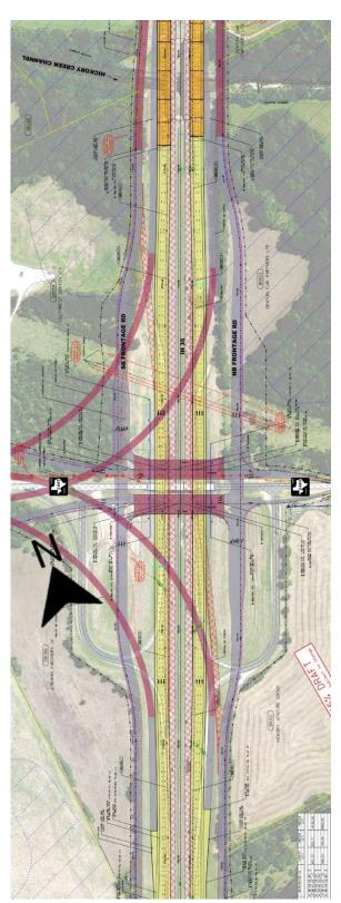
Future improvements to I-35W include new northand south-bound frontage roads which will require a realignment of the entrance and exit ramps to remove the current curved roadways to a more typical diamond pattern. The north-bound frontage road adjacent to the site will include a dedicated right-turn lane, one through-lane, one shared through and left-turn lane, one left-turn lane, and one u-turn lane (see graphic, left). Completion of improvements is anticipated for 2028.
