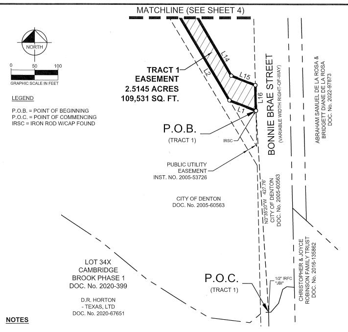
Bearing system based on the Texas Coordinate System of 1983 (2011 adjustment), North Central Zone (4202). A metes and bounds description of even survey date herewith accompanies this survey plat. The undersigned, Registered Professional Land Surveyor, hereby certifies that this survey plat accurately sets out the metes and bounds of the easement tract.
