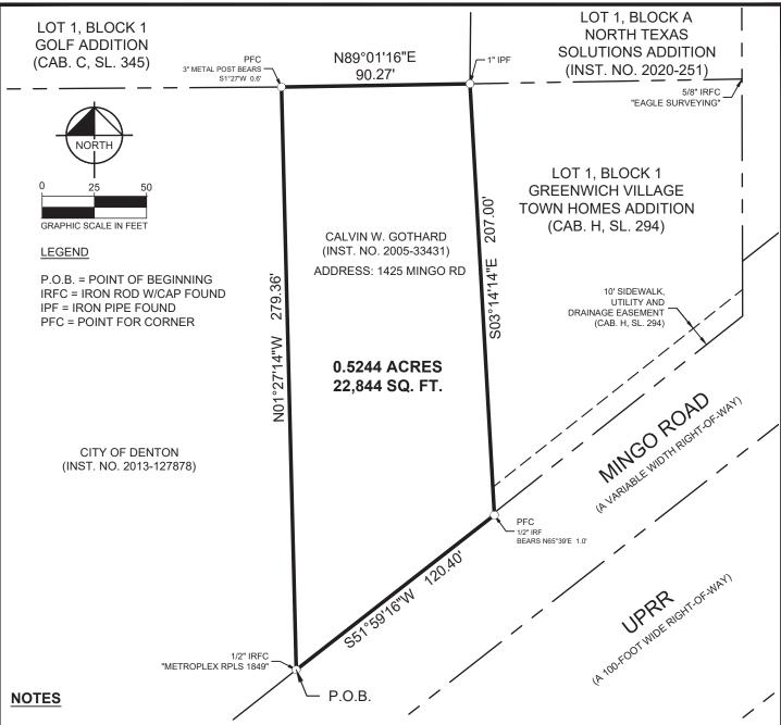
Bearing system based on the Texas Coordinate System of 1983 (2011 adjustment), North Central Zone (4202). A metes and bounds description of even survey date herewith accompanies this survey plat.
