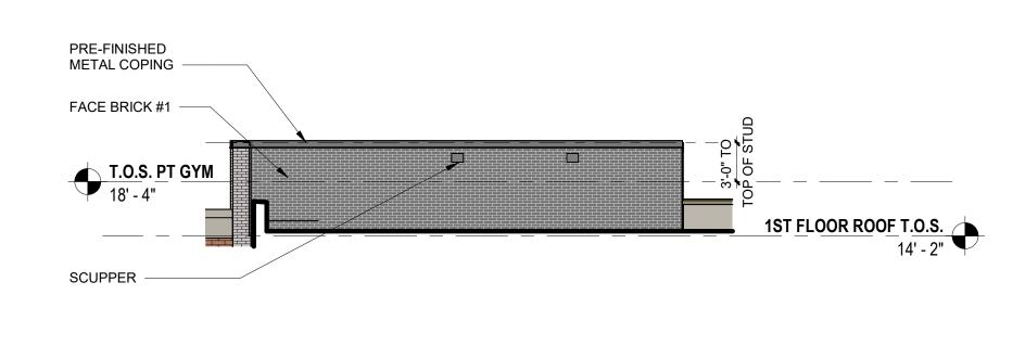
PREFINISHED METAL COPING -VERTICAL JOINTS EIFS #1 ON CMU -SEE SECTION FOR LOCATION OF HORIZONTAL JOINTS -FIRST FLOOR 4'-0" EQ. A EQ. A 4'-0" 24'-1 1/4"
