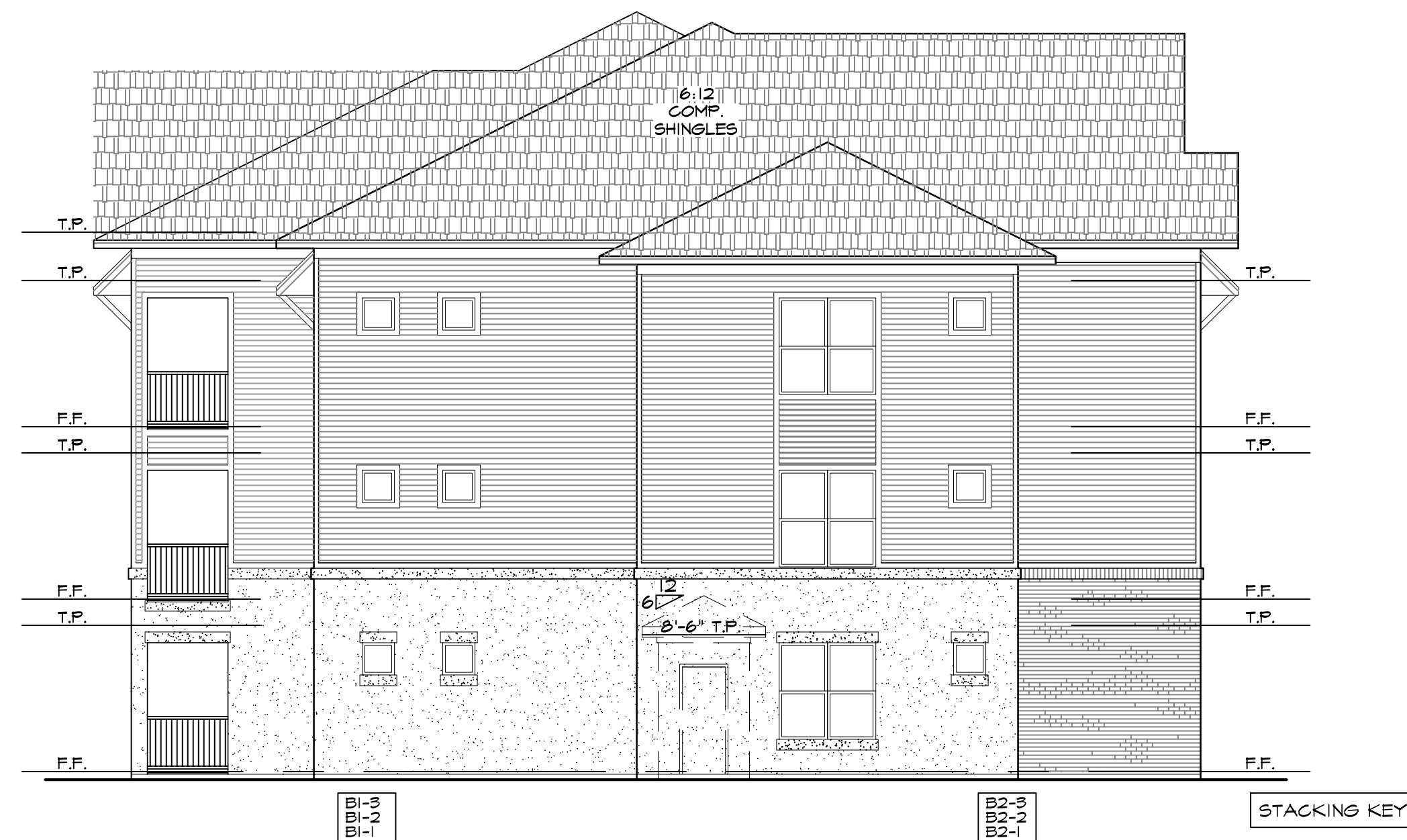
03 - RIGHT ELEVATION - BUILDING TYPE I-B
