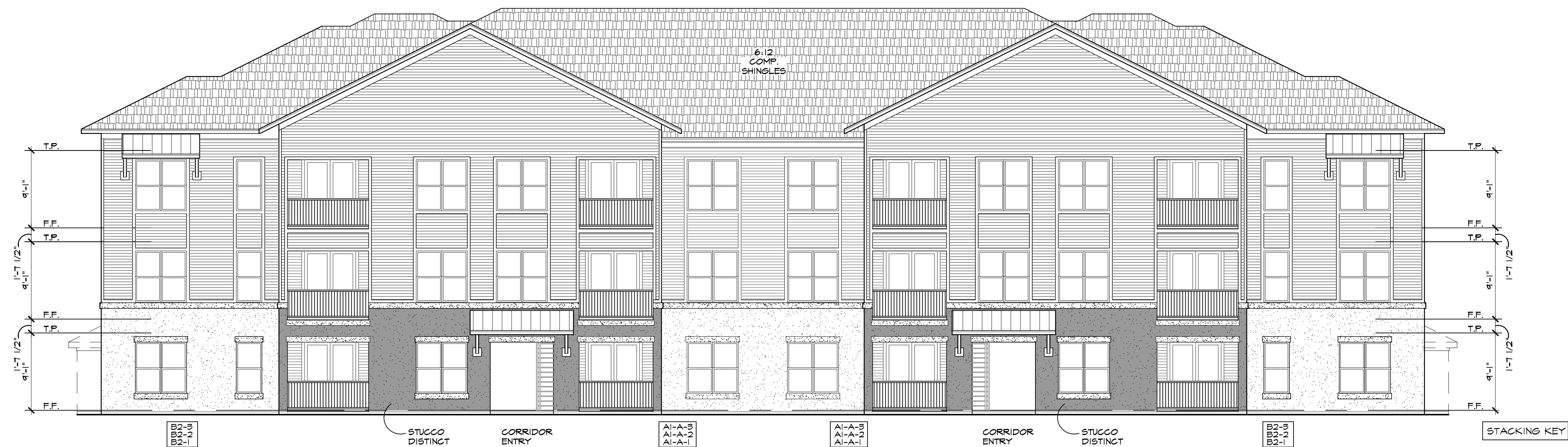
04 - REAR ELEVATION - BUILDING TYPE I-S
