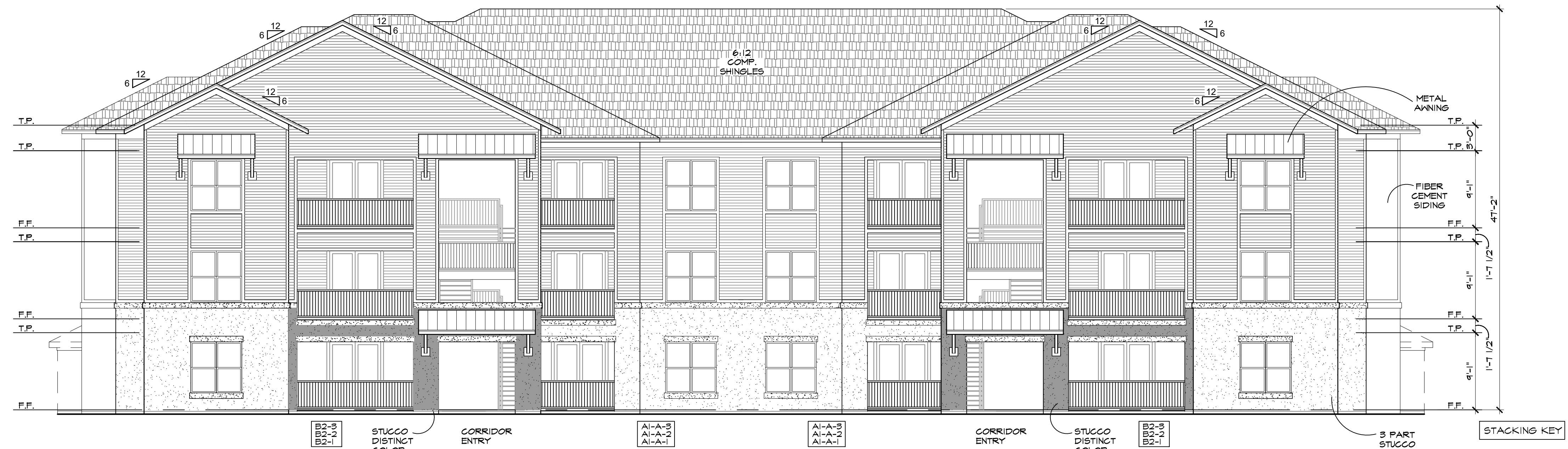
01 - FRONT ELEVATION - BUILDING TYPE I-S
